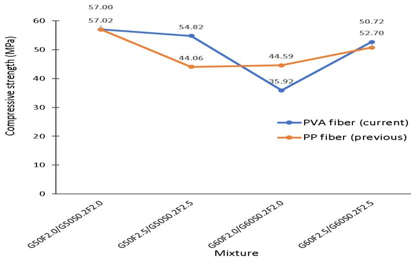
Figure 1. Comparison of compressive strength at 28 days
